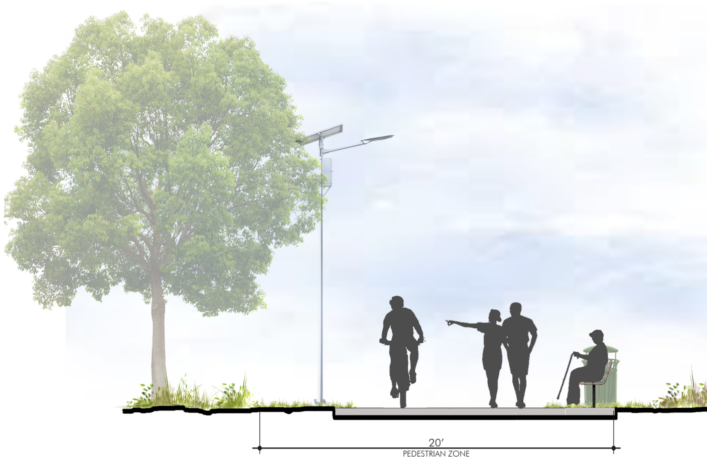
Prototypical trail section with ideal 20' wide pedestrian zone. Amenities may consist of 6' bike lane, 6' pedestrian lane, seating, lighting and buffer zones
